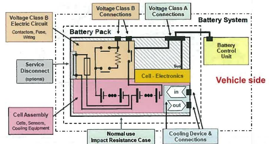
Figure 4 — Typical configuration of battery system with external BCU
