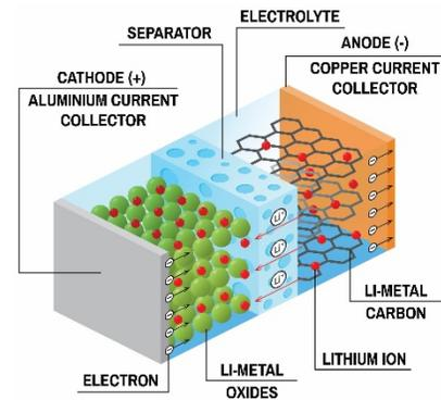
Image 3. Lithium-Ion Cell Discharging
